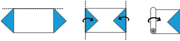
**To store the 4 Foot Skirt:** While in an indoor location with a clean, dry floor, roll the skirt on the floor with the vinyl side out and the cloth side in (**FIG. A**). Otherwise, to keep the 4 Foot Skirt off of the ground, simply roll the skirt with the vinyl side in as you are unsnapping the skirt from the bottom frame (**FIG. B**).
